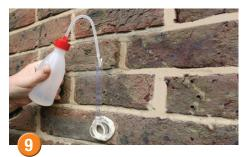
A Stormdry Gauge can be used to demonstrate the effectiveness of the treatment. The test should be carried out at least 28 days after applying Stormdry which allows the water absorption of the wall before and after treatment to be compared.
